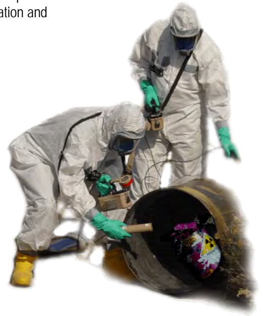
Surveying an actual Radiological Exposure Device (RED) in a contaminated area during a training exercise
